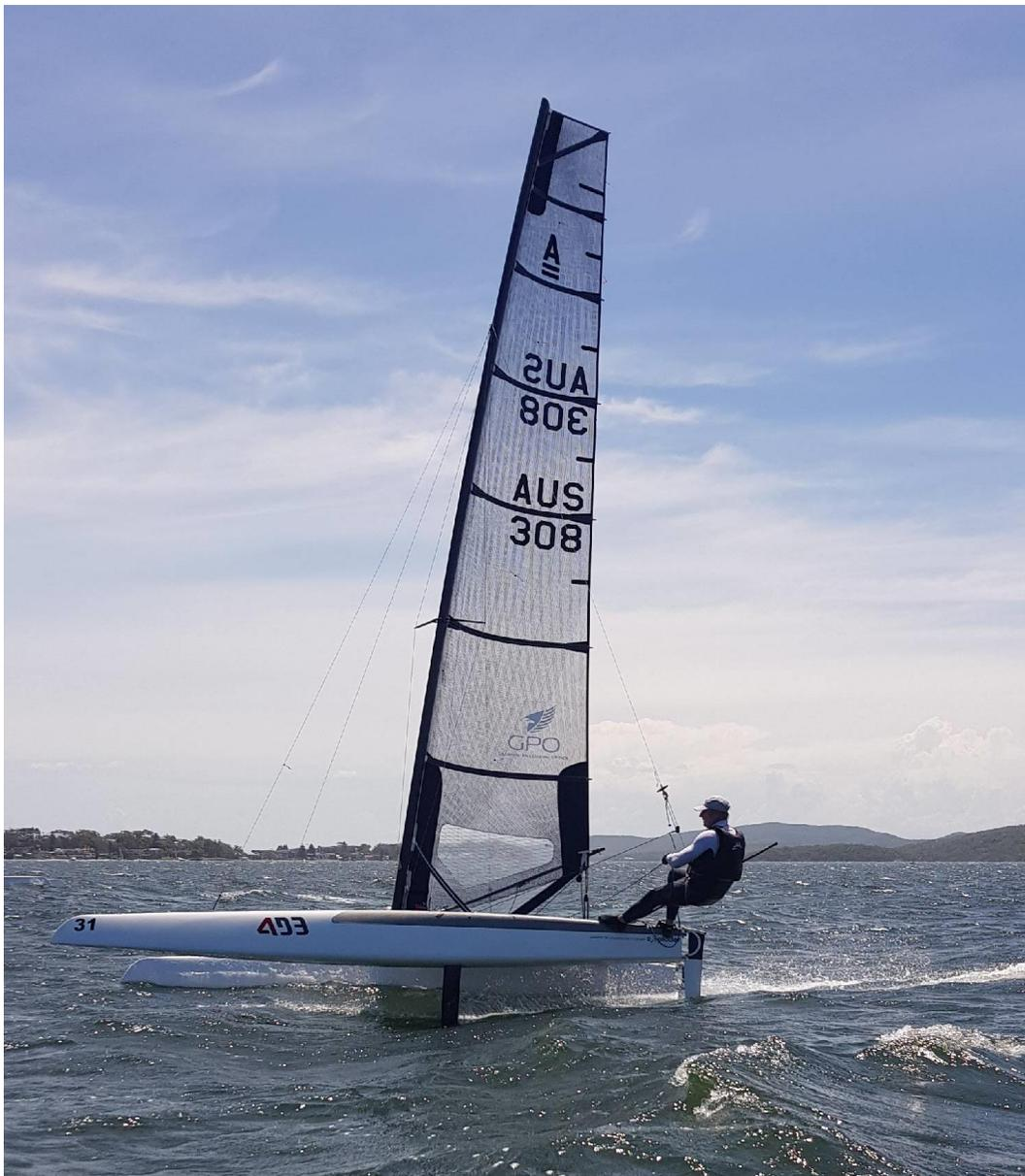
The reason for this is that there is such a huge difference between having foils that lift and actually foiling fast. The foiling boats appear extremely difficult to get up and stay foiling, but when they do foil, the performance difference is massive. Downwind, especially in moderate conditions this is most noticeable. Upwind the foilers are very fast in a straight line, but also sail very low, so their true gains are not as clear.
